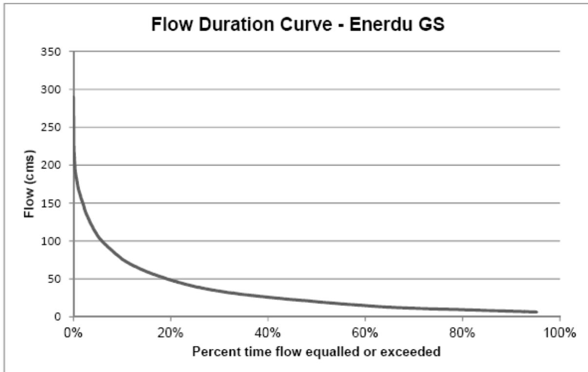
The Flow Duration Curve shows that a flow of 42 m<sup>3</sup>/s is available less than 25% of the time. It seems uneconomic to design a facility of this capacity that will operate at full capacity for less than 25% of the time.
